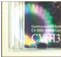
Without polarization filter The CD case reflects the illumination.
