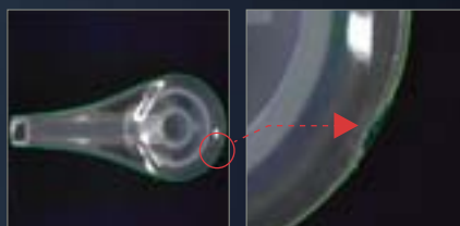
Detection of minute flaws along the profile
