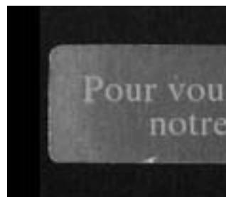
The glossy background of the label appears dark and the print appears bright.
