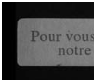
The glossy background of the label appears bright and the print appears dark as it diffusely reflects the light.
