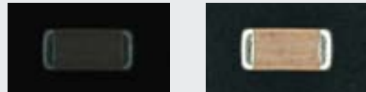
Image comparison at a shutter speed of 1/10,000 sec. (both images shot under the same conditions using fluorescent lighting.)
