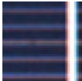
■ 310,000 pixels Lines are out of focus and cannot be detected.
