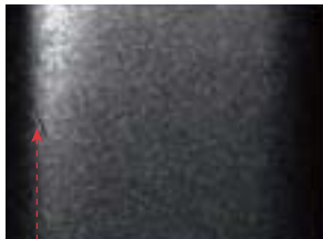
Normally, the dent in this image could not be detected because of the random glare and granular texture of the metal.
