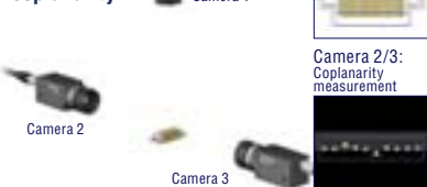
Simultaneous measurement of pitch and coplanarity
