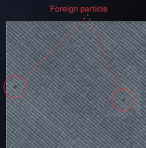
Foreign particle detection on diagonal striped background
