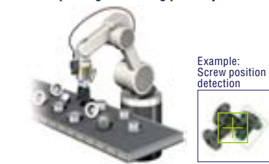
Random picking of bushing parts by robots
