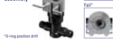
Checking for missing O-rings or O-ring misalignment during EGR valve assembly
