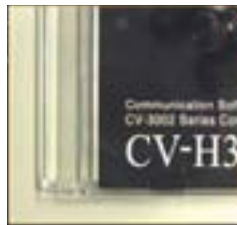
With polarization filter The polarization filter reduces the reflection.
